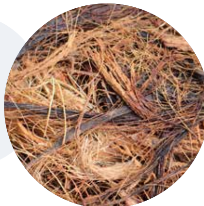
Flax fibre, coconut shells and agave fibres are examples of plant-based raw materials that we use in RheVision, our biofibre-reinforced polypropylene series.
